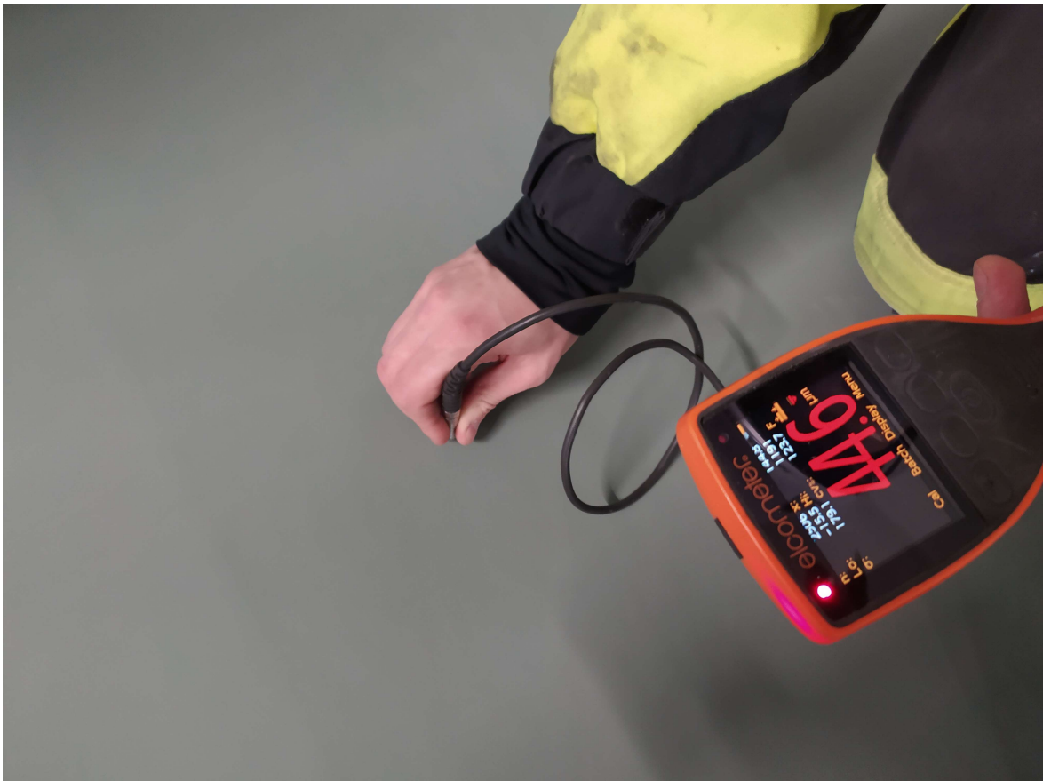
Figure 9: Author measuring first layer film thickness on inspection
