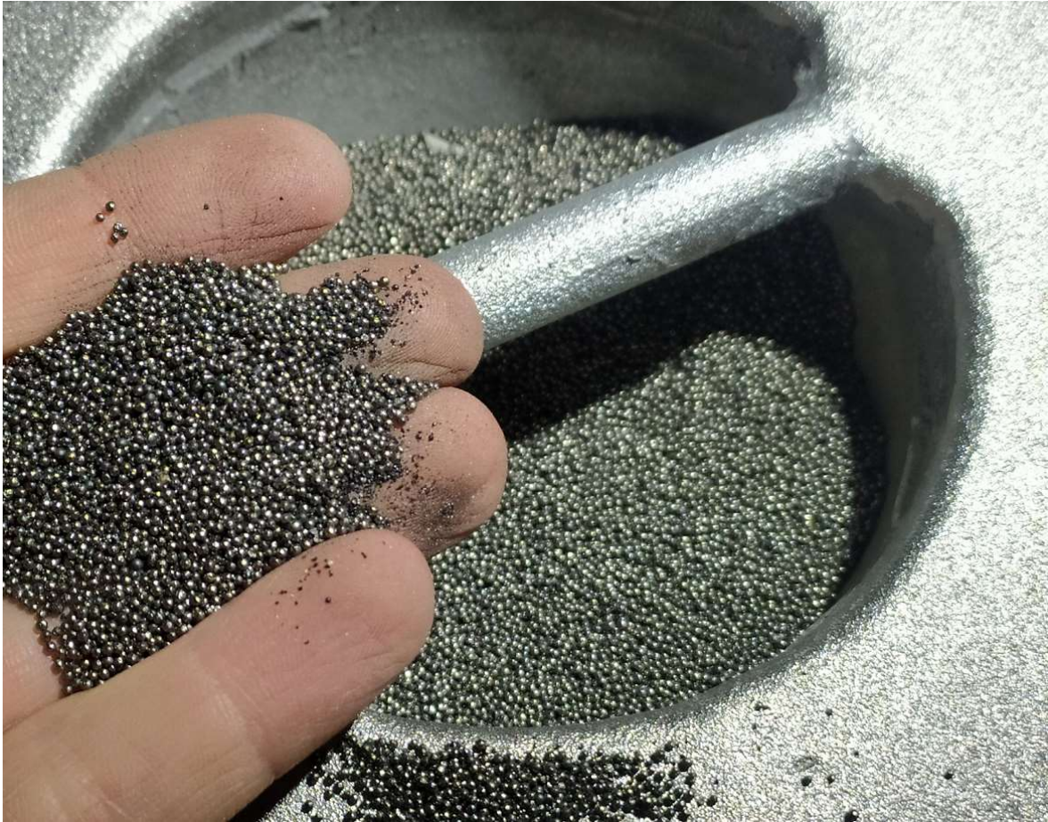
Figure 5: Metal particles used for blasting. Freshly blasted area on background.
