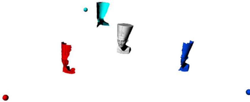
Figure 10. Scanning of object of interest from different viewpoints (Wujanz & Neitzel 2016, 6).
