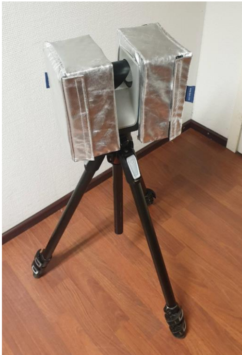
Figure 21. Faro Focus equipped with cooling elements.
