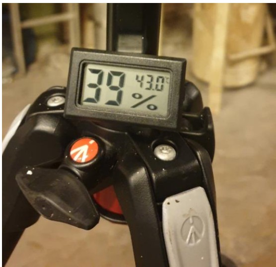
Figure 27. Atmospheric conditions at mezzanine level.
