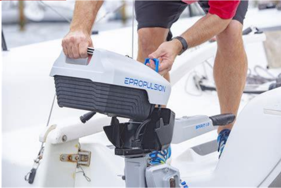
Figure 5. 2 Integrated Battery installations in electric outboard motor (ePropulsion.com)
