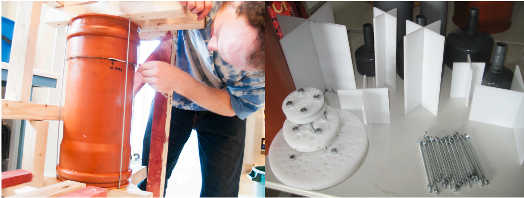
Figure 6. Left: Assembled wide (190mm inner diameter) filter with the custom made end cap. Keiran is pushing the Teflon tape, which moves during sealing back into the cracks to stop leakage.
