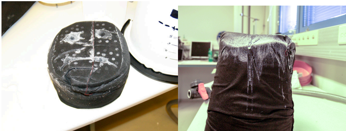
Figure 24. Left: Compression from the fastening nut has visibly increased deposits of test dust (the two eyes and corner of the mouth). Spots reveal the placement of the holes in the displacer. The bag dimensions were not optimal as can be seen from the visible creases.
