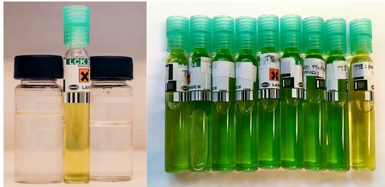
Figure 26. Left: GAC9 sample with pre-filter water sample on the left, reacting LCK 304 Ammonium sample cuvette (LANGE, USA) in the middle and post-filter water sample on the right.
