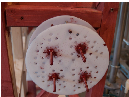
Figure 8. Epoxy coated 190 mm dispersers on the test rig.
