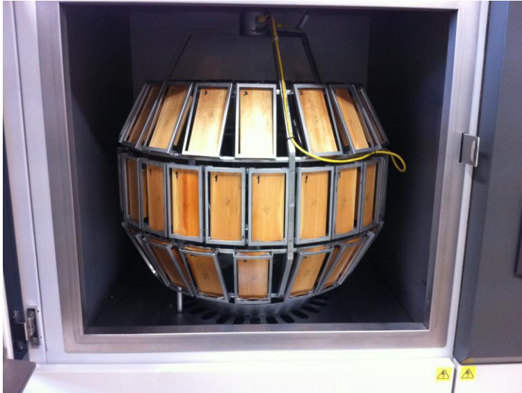
Figure 12. Positioning of test specimens in the Ci4000 Xenon Weather-o-meter
