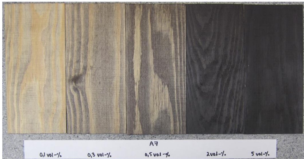
Figure 18. Coating A7 with different volume concentrations (0.1 vol-%, 0.3 vol-%, 0.5 vol-%, 2 vol-%, 5 vol-%)
