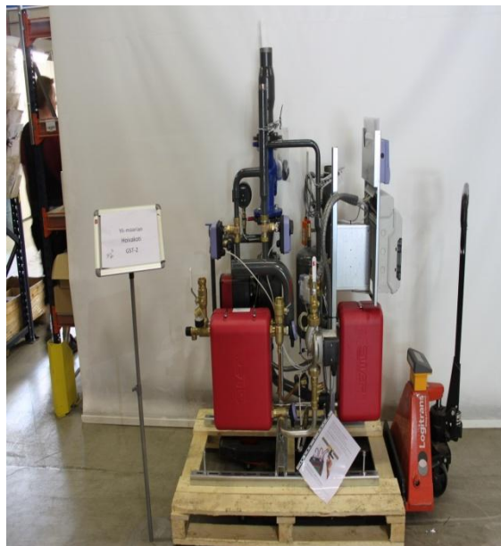
FIGURE 3. Two step connection heating substation, DN 32, safety valve, and service valve, substantially standard
