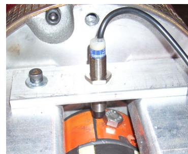
Illustration 4: tach sensor on our dyno
