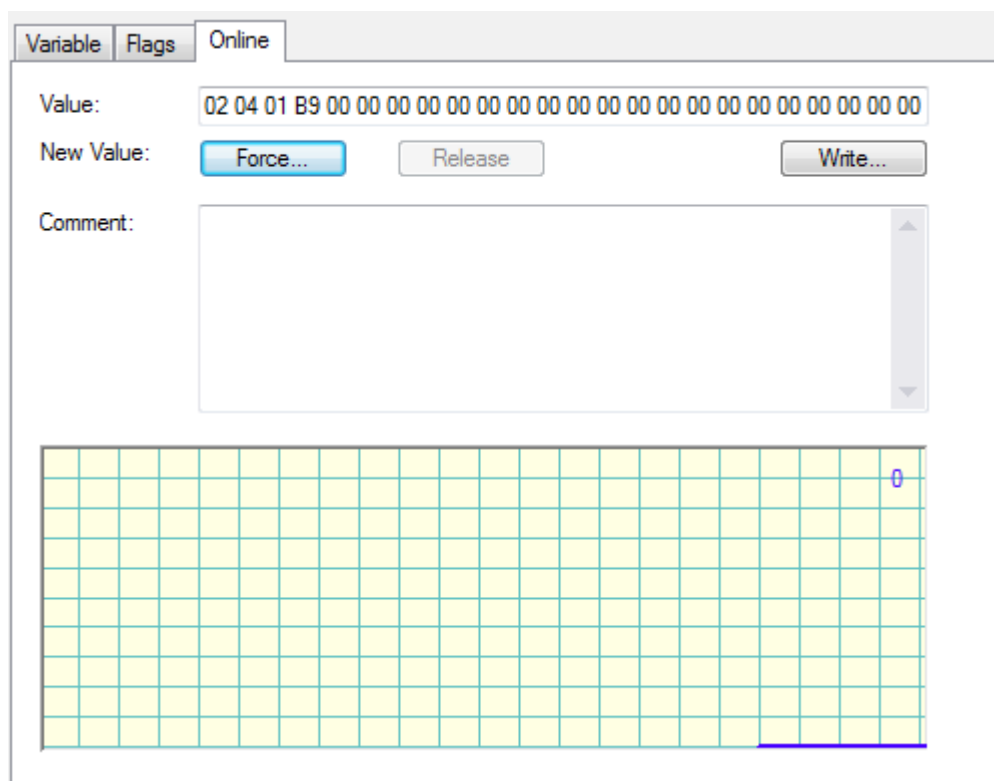
Figure 16: PROFINET input message shown as hexadecimals in TwinCAT
