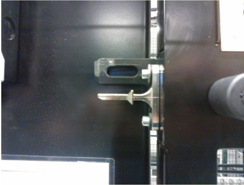
Figure 19 Improved latch in place.
