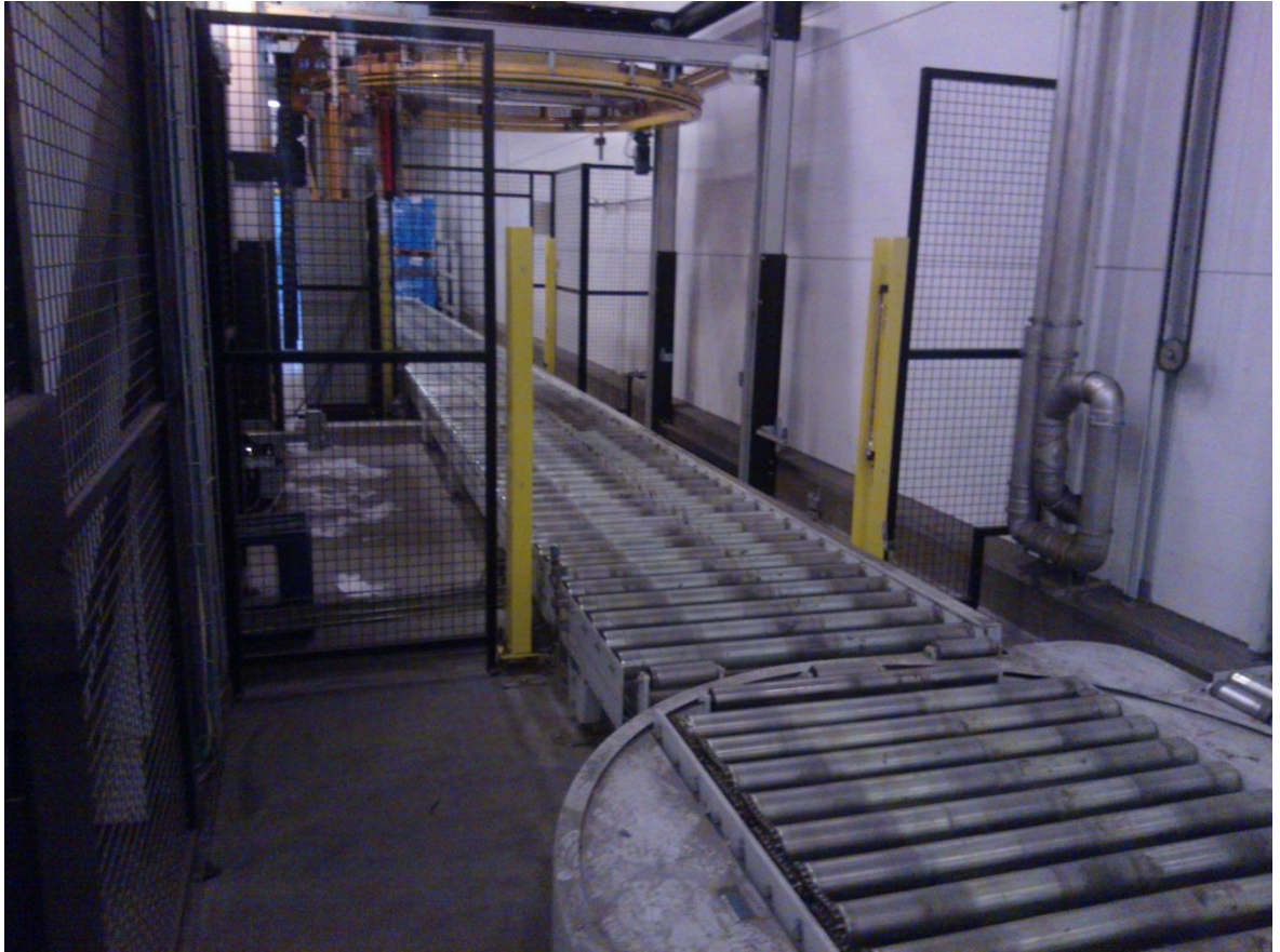
Figure 9 Pallet wrapping machine's safety light grids (four yellow posts, two at front and two further behind the wrapping machine).
