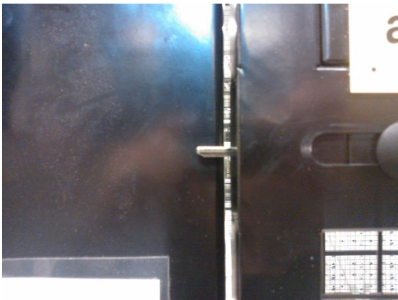
Figure 16 Safety switches actuator key may hit to the door frame.
