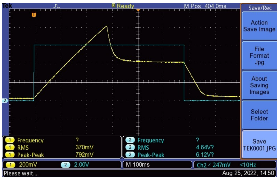
Figure 10: Envelope generators full cycle measured with an oscilloscope
