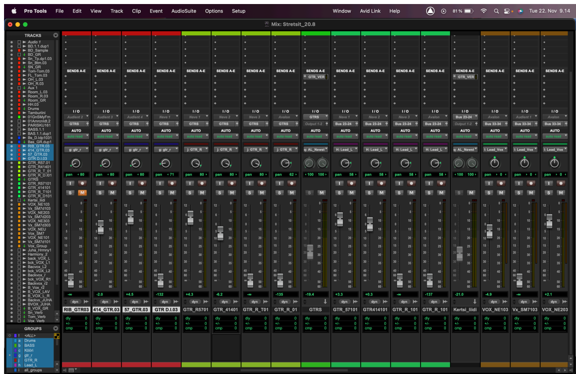
PICTURE 7. The guitar tracks in Pro tools on the left highlighted in red colour. The Ribbon microphone track, AKG 414 track, Shure 57 track, and D.I. track. (Pöllänen 2020)
