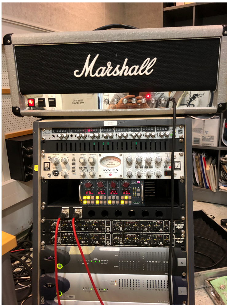
PICTURE 6. One signal (red XLR cable on the right) going from DI Box into the Neve Preamp, and the other signal (black guitar cable) going into the input of a Marshall amplifier. (Pöllänen 2020)
