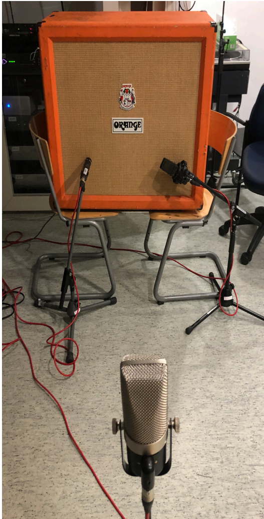
PICTURE 8. Microphone setup clockwise from top left: Shure SM57 dynamic microphone, AKG C414 condenser microphone, A.I.R Peacemaker ribbon microphone. (Pöllänen 2020)
