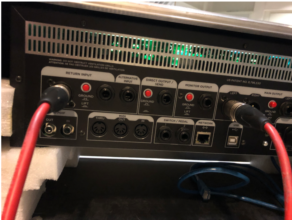
PICTURE 10. Connecting the D.I. signal to Kemper return input and taking the processed signal out of the Kemper from the main output. (Pöllänen 2020)
