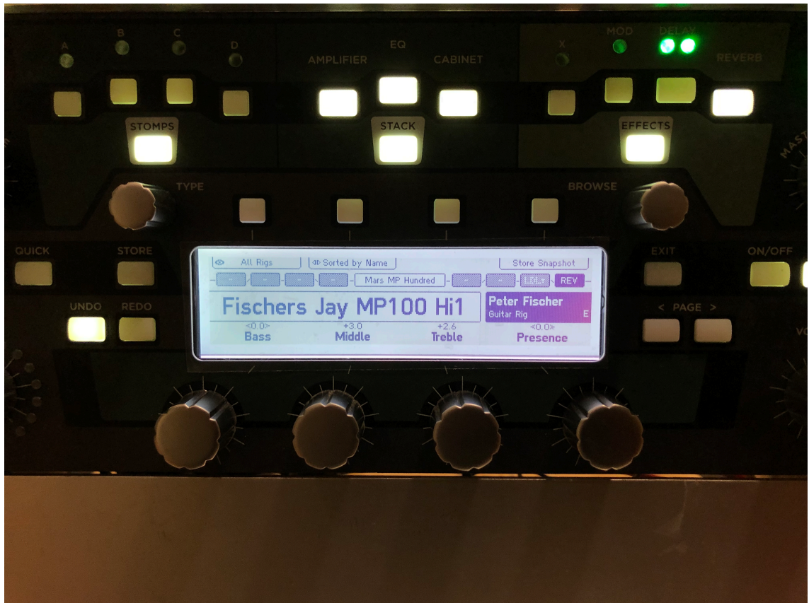
PICTURE 12. Selecting the rig to reamp with on the Kemper Profiler (Pöllänen 2020)
