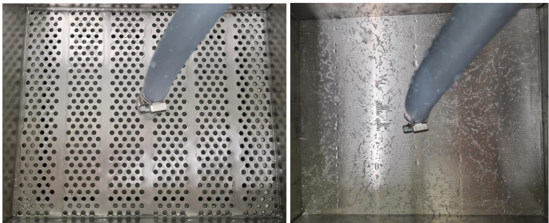
PICTURE 31. Examples of coarse and fine rejects on tested MF-liners. (Reisinger, 2022)
