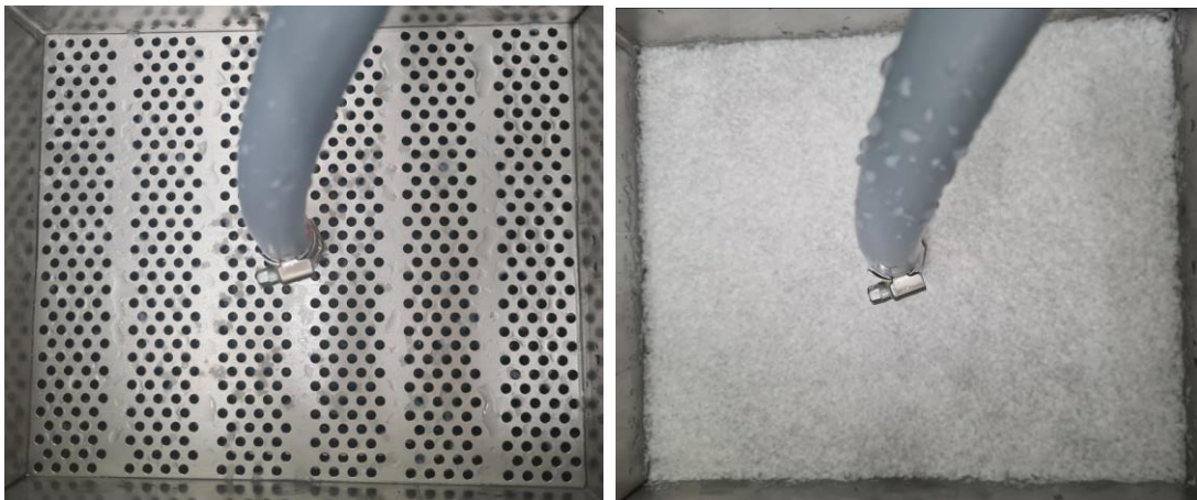
PICTURE 25. Example of coarse and fine reject typical for two side siliconized glassines. (Reisinger, 2022)
