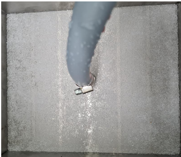
PICTURE 21. An example of fine reject on the filter after fractionating. (Reisinger, 2022)
