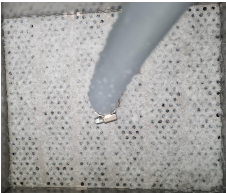
PICTURE 19. An example of coarse reject on the filter after fractionating. (Reisinger, 2022)
