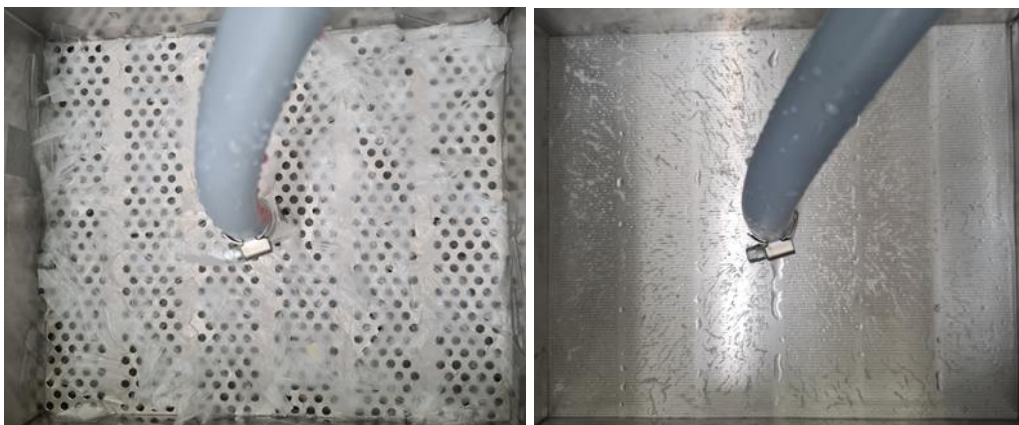
PICTURE 29. Examples of coarse and fine rejects on tested PE-liners. (Reisinger, 2022)
