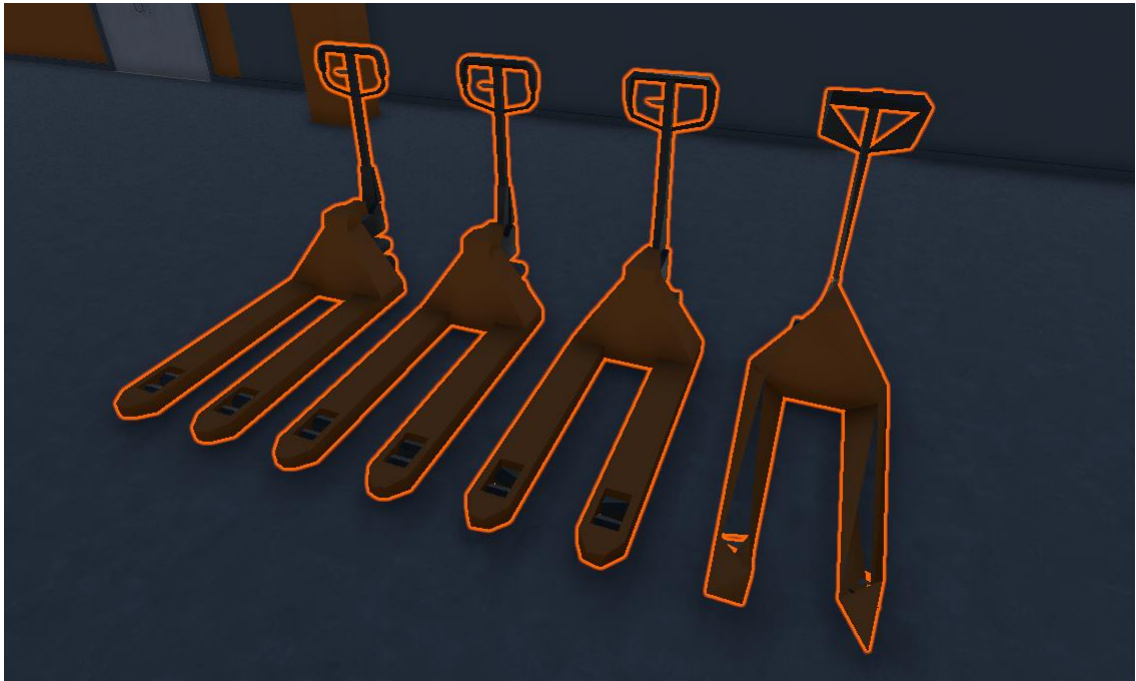
Picture 12. From left to right. Different LODs of the same object decrease in detail inside Unity.
