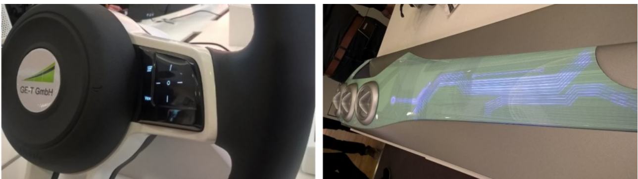
PHOTO 1. Structural electronic products for the automotive industry. Car steering wheel with embedded functionalities (left) and car dashboard element with embedded electronics (right) (photos: Tomi Tuomaala).
