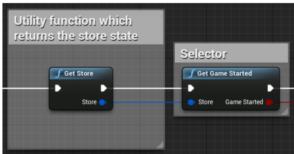
Image 28. Store state structure received from a utility function is passed to a selector.
