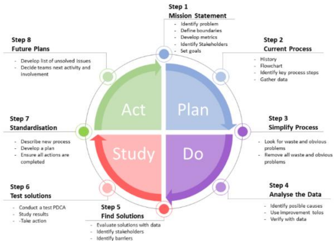
FIGURE 15. Eight steps for PPI, PDSA-cycle-based. from A Plan-Do-Check-Act Based Process Improvement Intervention for Quality Improvement Jorge Luis Garcia-Alcaraz.
