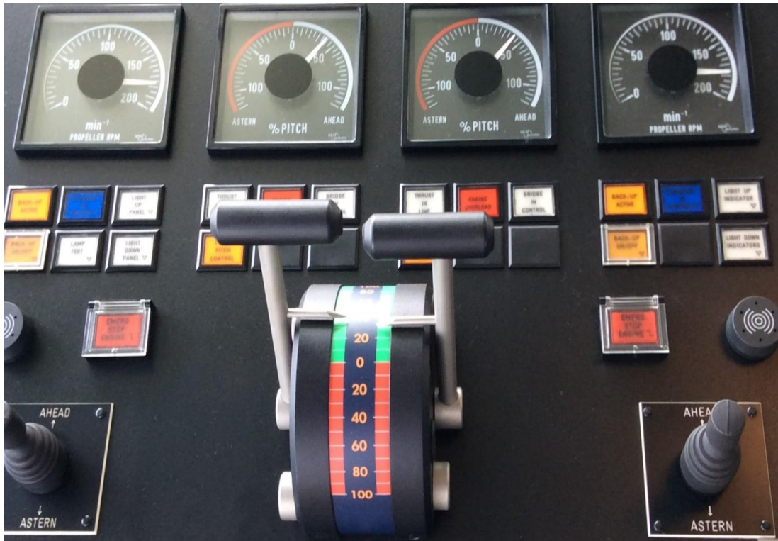
Figure 21. Pitch controls and various indicators, MV MERSol (Koivisto, 2015)
