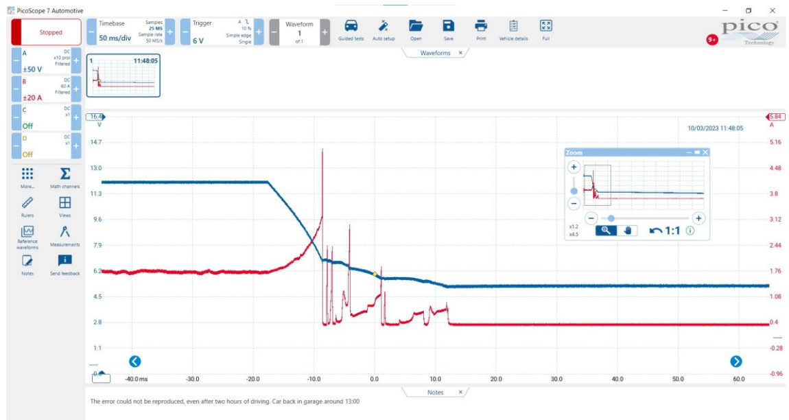
Figure 15. Voltage and current measurement while powering out a lidar sensor.
