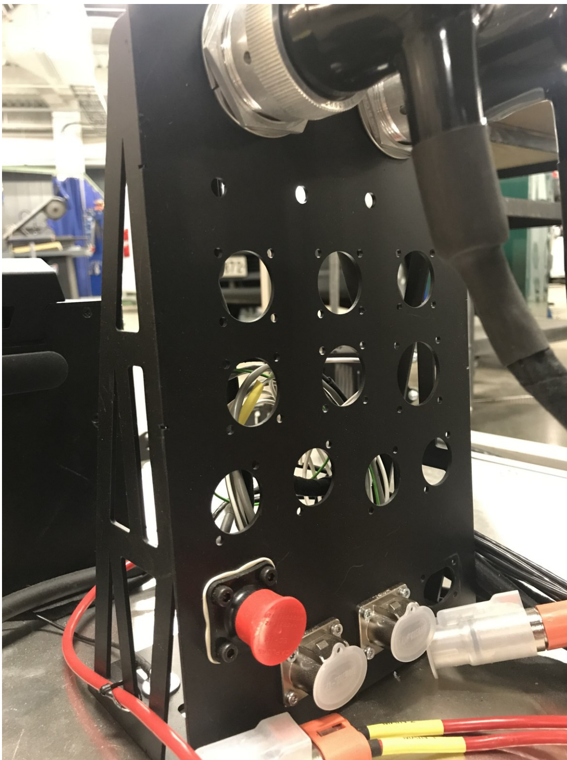
Figure 11. Test Bench Connection Panel being made.
