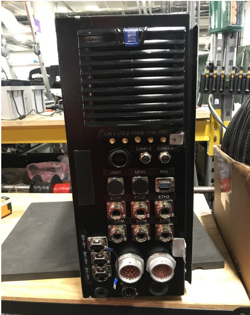
Figure 12. Toyota Proace AD-box including the computing unit's front cover with the connectors.
