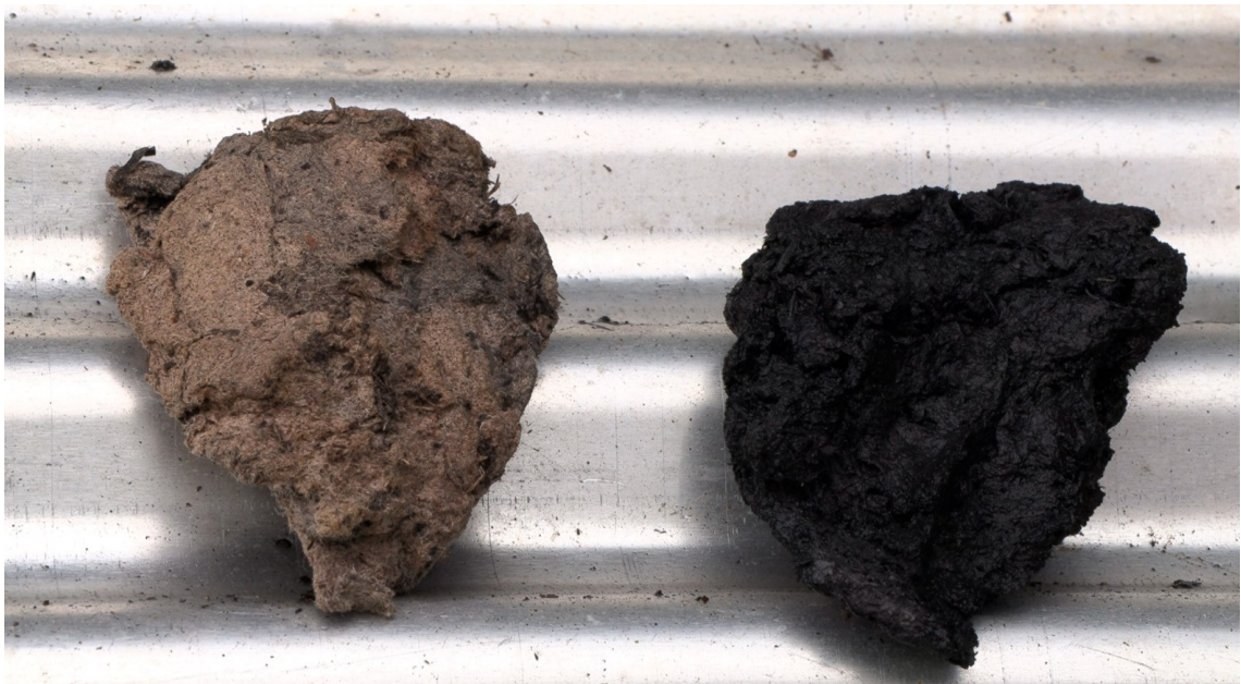
PICTURE 7. Piece of zero fibre and pyrolyzed biochar. Photo by Isa Kiviaho.
