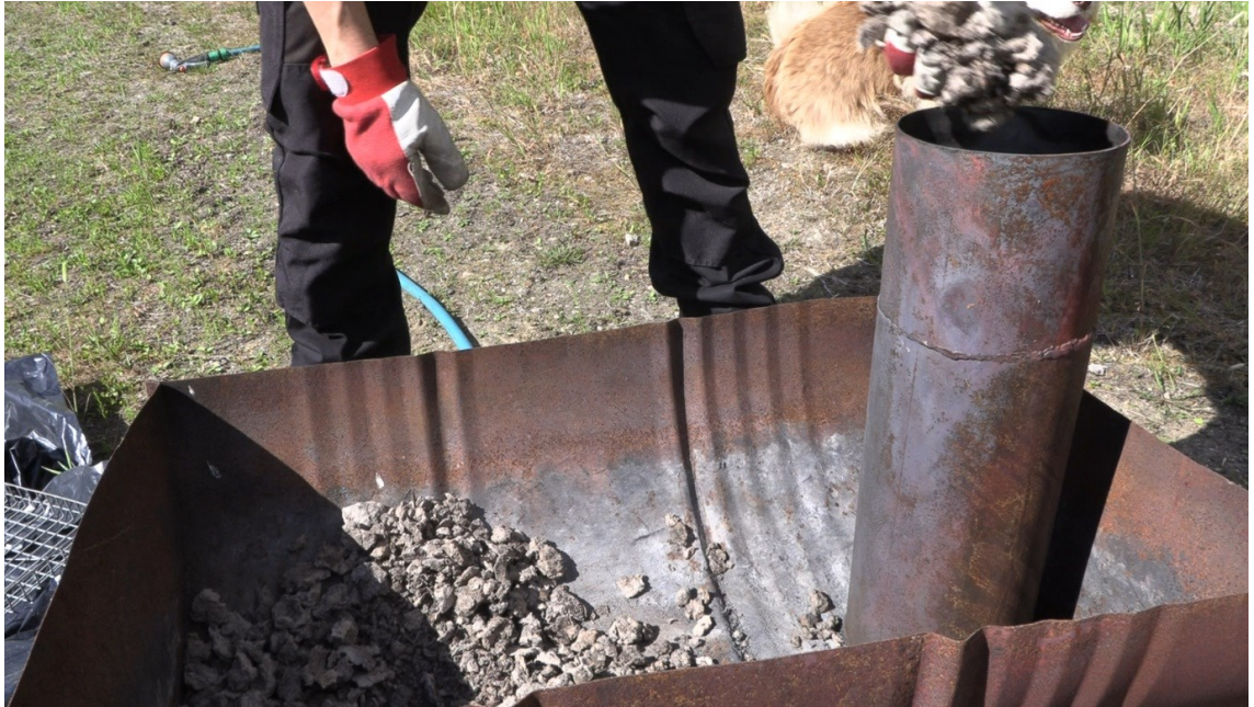
PICTURE 2. Setting dry zero fibre in pyrolysis. 8.7.2022. Photo by Isa Kiviaho.
