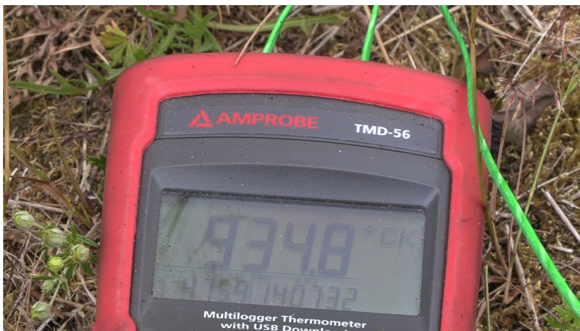
PICTURE 5. Temperature record in pyrolysis. Photo by Isa Kiviaho.
