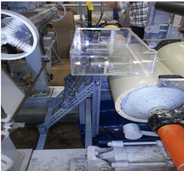
FIGURE 13. Size box and bracket installed
