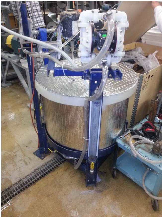
FIGURE 16. Insulated day tank with drain and drawdown tube
