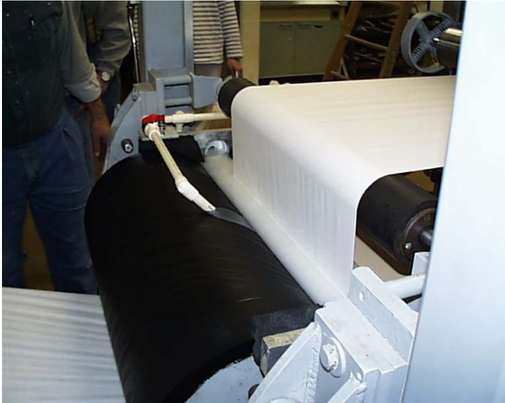
FIGURE 8. Original pond size press design at UWSP paper machine
