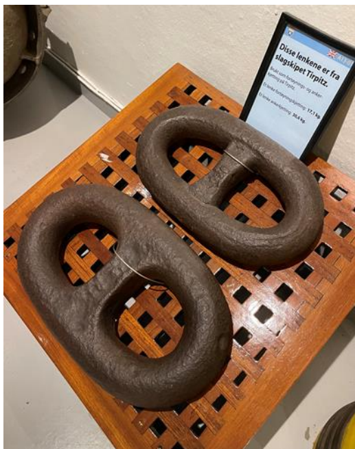
Figure 5: Common (17 kg) and enlarged stud links (30 kg) (Wolfmann, 2021).
