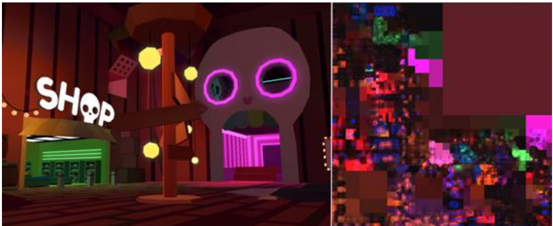
PICTURE 23. On the left of the image is the lobby scene in Unity using baked lights. On the right is the final Lightmap texture.
