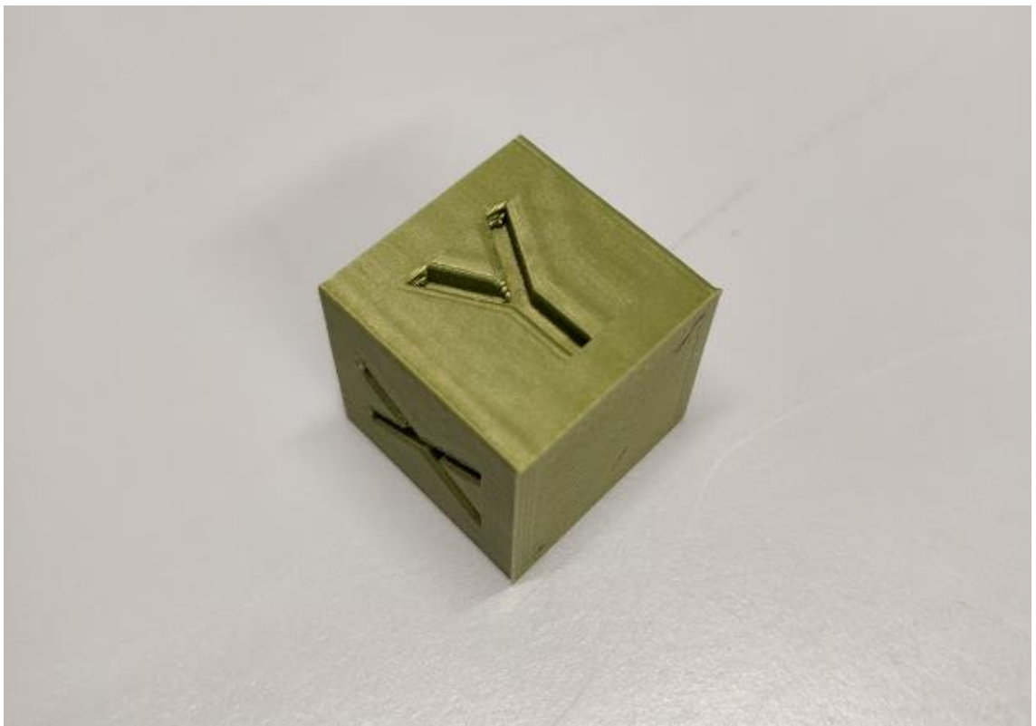
Figure 40. Ghosting due to vibrations
