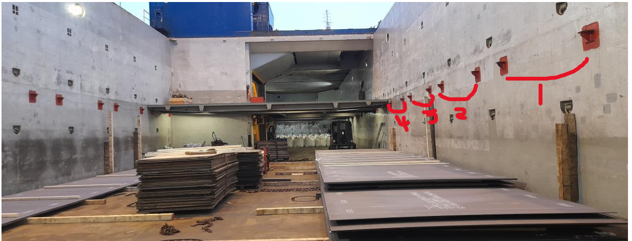
Figure 24: 4 plates from the tween deck were removed in order to load the steel plates.
