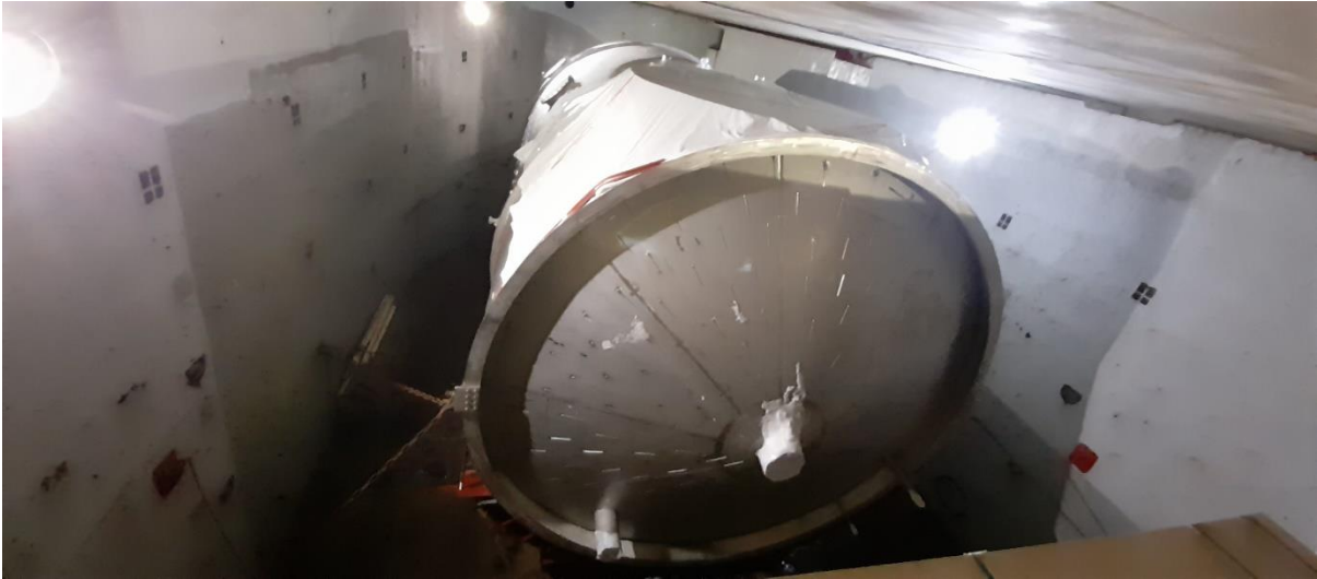
Figure 30: Scrubber special project cargo loaded and secured for sea.
