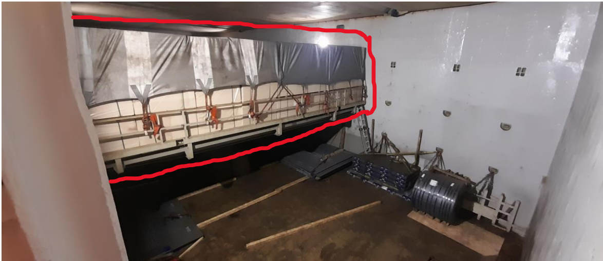
Figure 14: Plywood loaded on tween deck and secured with tarpaulin for sea.
