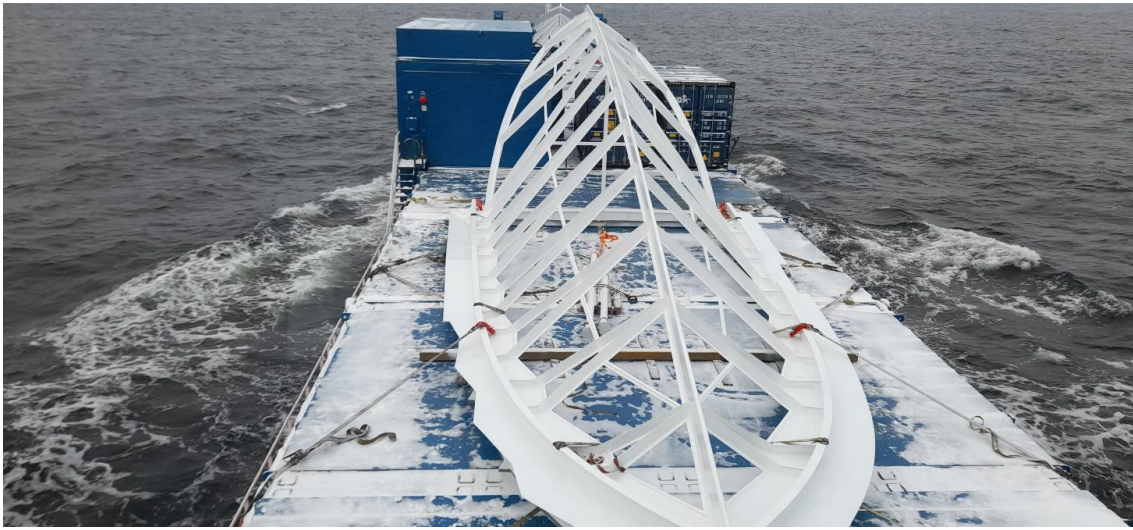
Figure 27: special project cargo secured on top of hatch cover.
