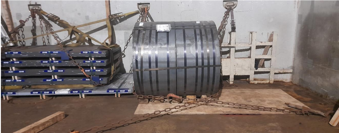
Figure 11: Steel coils secured with chains and speed lashes.
