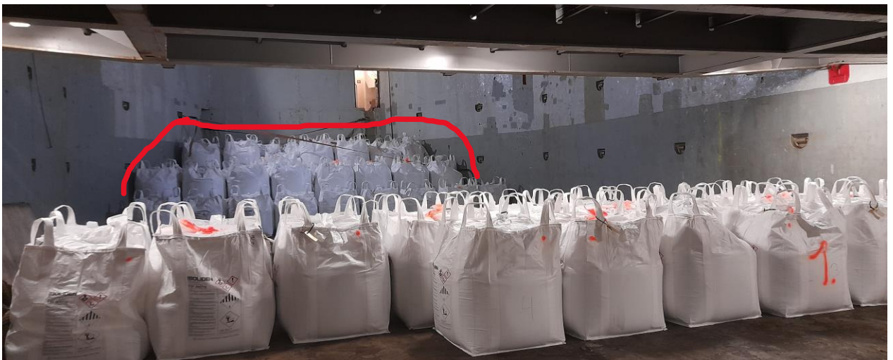
Figure 23: 3 high stacks of nickel matte in big bag on tank top. 08-12-2022
