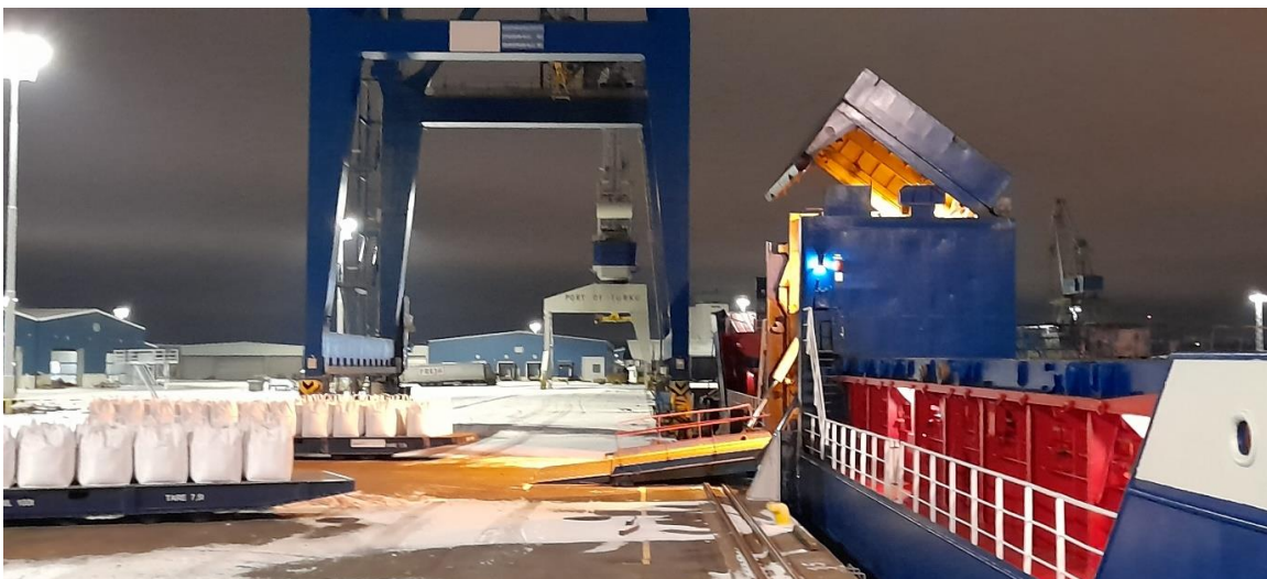
Figure 21: side loader or Side lift Loading of Nickel matte in big bags (IMO class 9), Turku 22-11-2022
