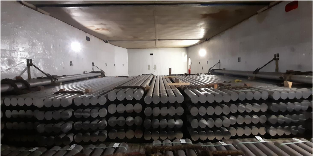
Figure 26: Alu logs loaded and secured on tween deck.
