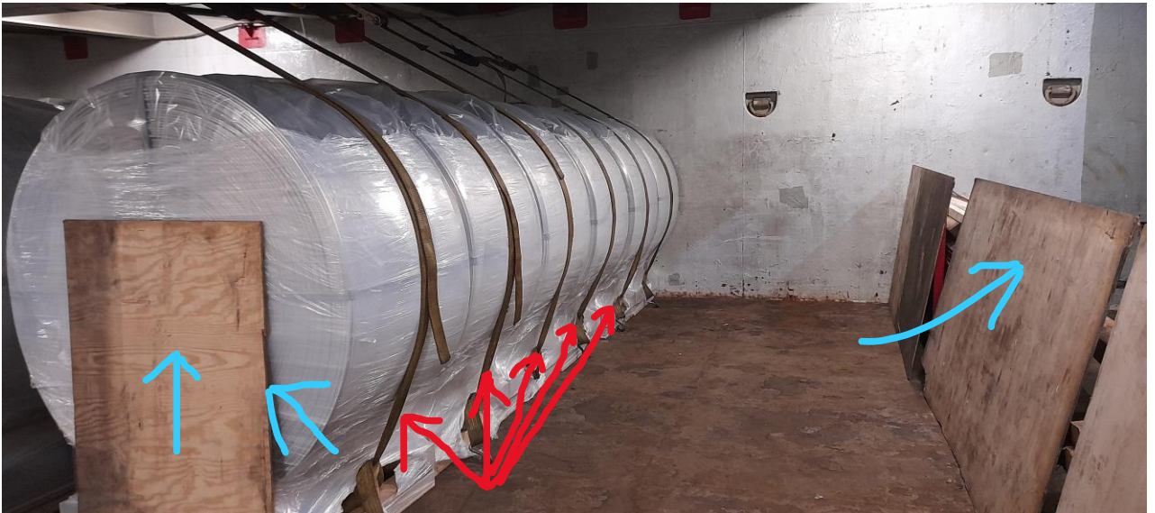
Figure 20: Aluminium wire rod coils secured with ratchet straps from tween deck to tank top.
