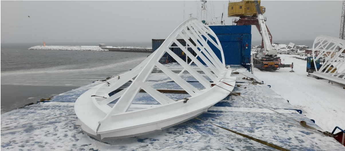
Figure 28: Special project cargo DINO frame secured on top of the hatch covers.
