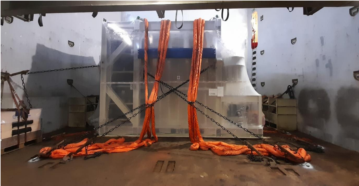
Figure 32: Transformer secured with chains and speed lashes.
