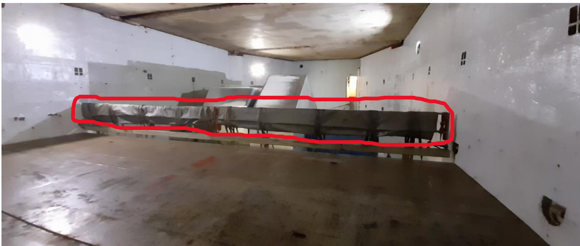
Figure 8: Tarpaulin is well prepared and tween deck is ready for cargo.
