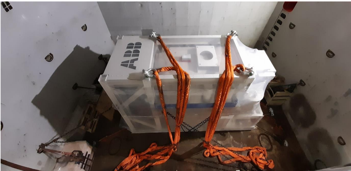
Figure 31: Special project cargo Transformer secured on tank top cargo hold aft.
