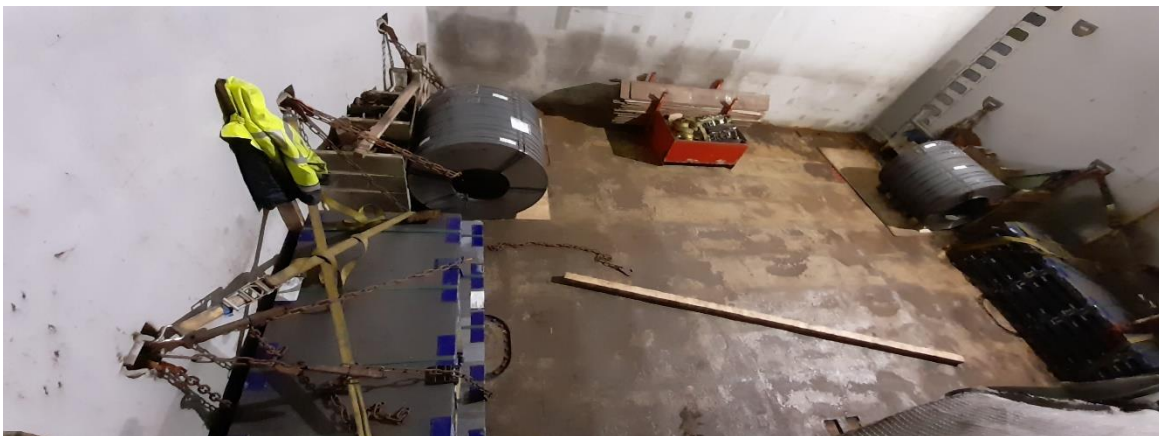
Figure 12: Steel coils loaded and secured on tank top, in cargo hold (on tank top).
