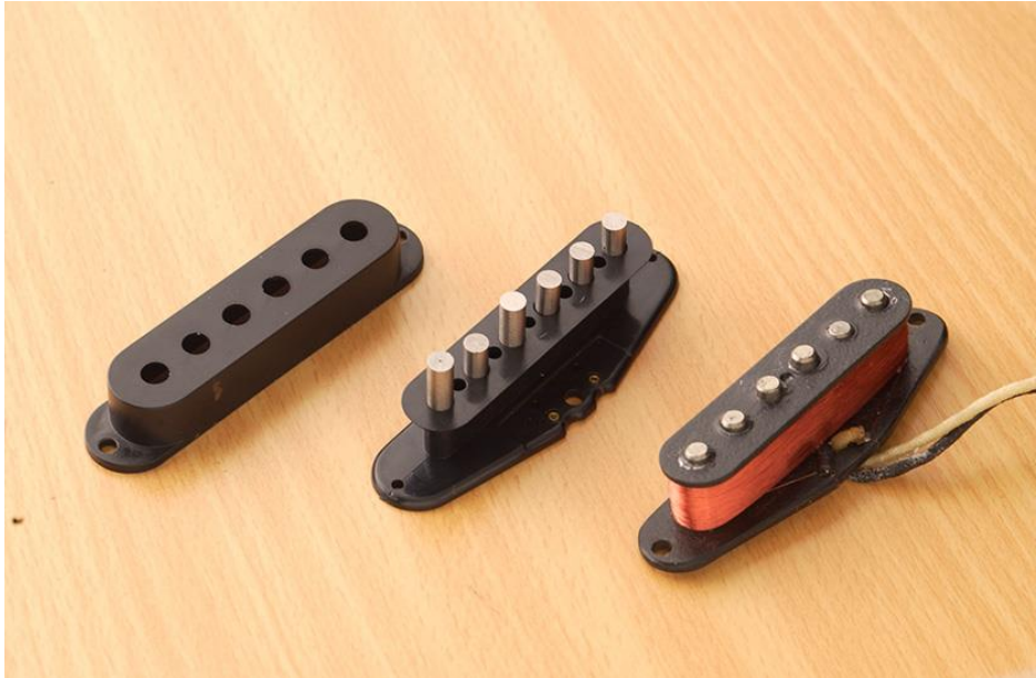
Figure 15. Construction of Magnetic Coil Pickups [19].
