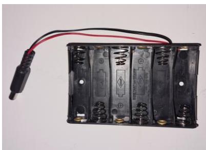
Figure 11. Standard 2.1mm pin, 9V battery pack.
