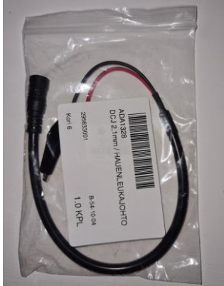
Figure 12. 2.1mm DC power plug attachment.
