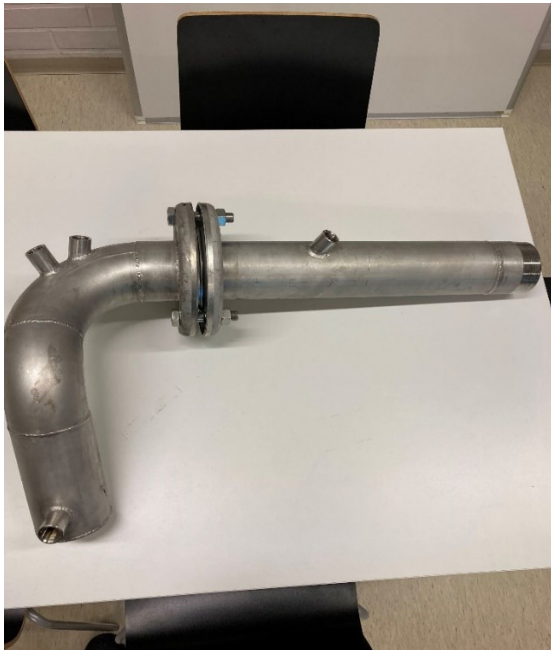
Figure 21. Reactor pipe with bend
