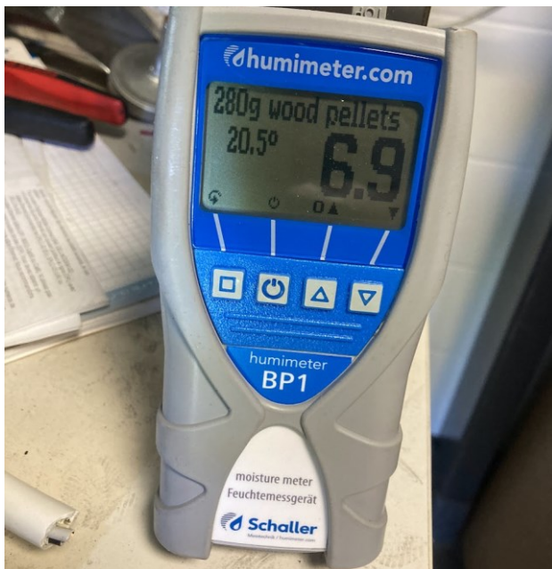
Figure 15. Humimeter BP1 measuring the moisture of 280 grams of wood pellets
