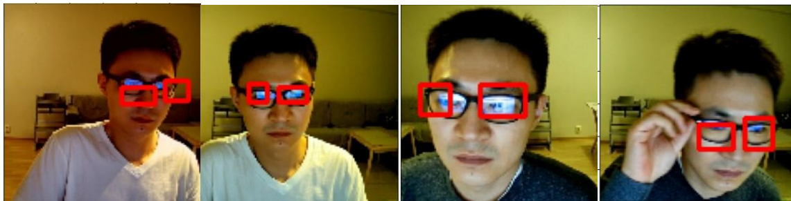
Figure 18. Predicted bounding boxes by customized MobileNetV3
