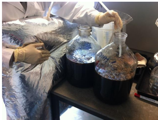
FIGURE 10: Injecting pure Nitrogen to the batch reactor
