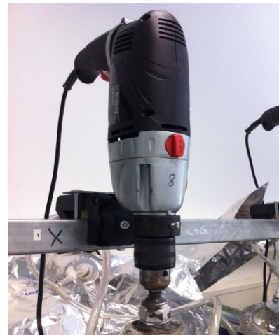
FIGURE 14: Stirring device made from drill
