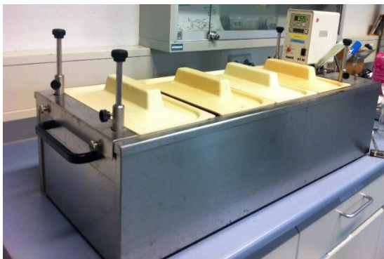
Figure 23: Water bath for 70 Celsius degree sanitation
