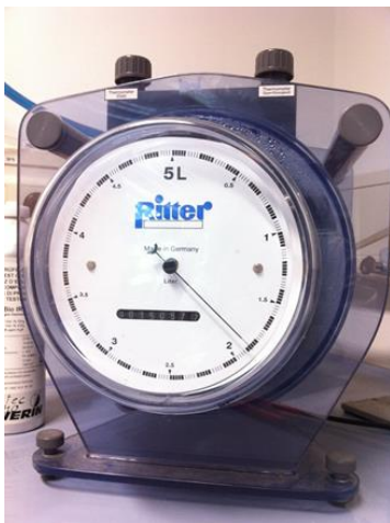
FIGURE 29: Ritter gas meter
