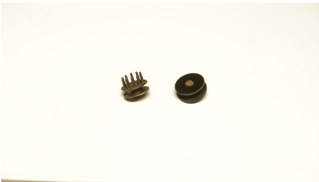
Figure 6. Original Enobio Multiplestuds (left) and flat (right) electrodes
