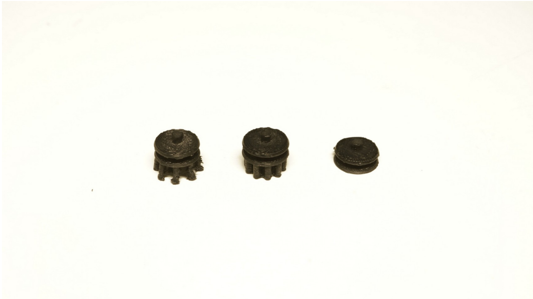
Figure 30. Headpin Spiderman (left), MultipleStuds (center) and flat (right) electrodes printed with FilaFlex conductive material and Electrically Conductive Paint
