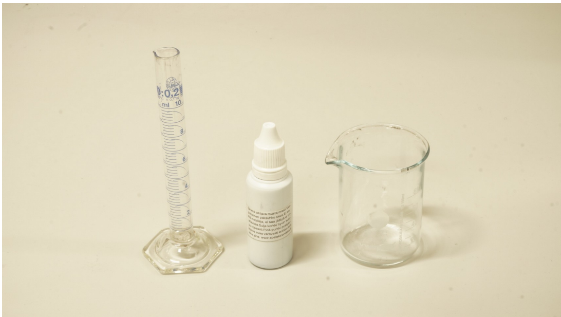
Figure 13. Electrically conductive paint and tools used for diluting it in 100 drops of water
