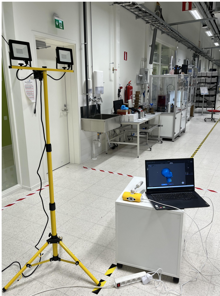
Figure 1. Set up for 3D scanner with CreaLity CR-Scan Lizard 3D scanner and CR-Studio software
