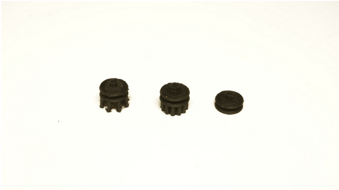
Figure 8. Headpin Spiderman (left), MultipleStuds (center) and flat (right) electrodes printed with FilaFlex conductive material
