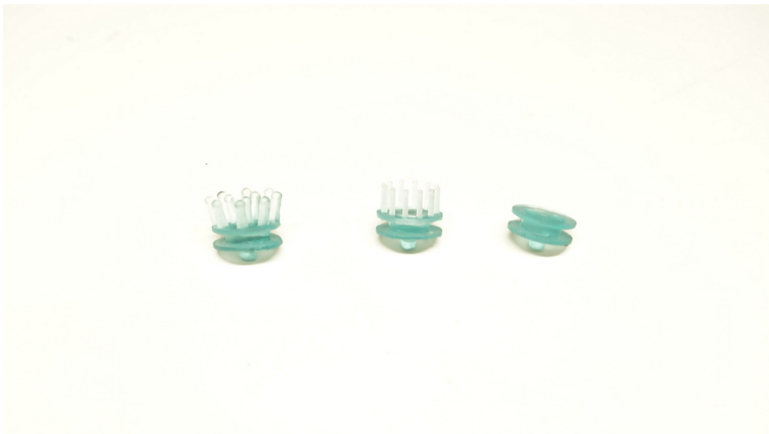
Figure 11. Headpin Venom (left), MultipleStuds (center) and flat (right) electrodes printed with Siraya Tech Blu material
