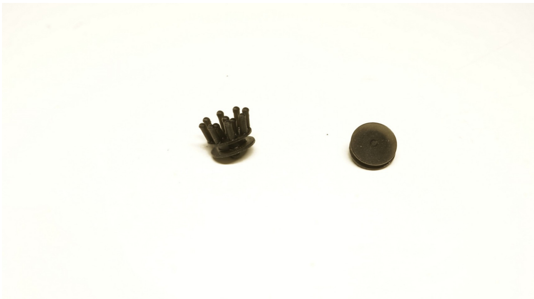
Figure 12. Headpin Venom (left) and flat (right) electrodes printed with Resione F80 resin material
