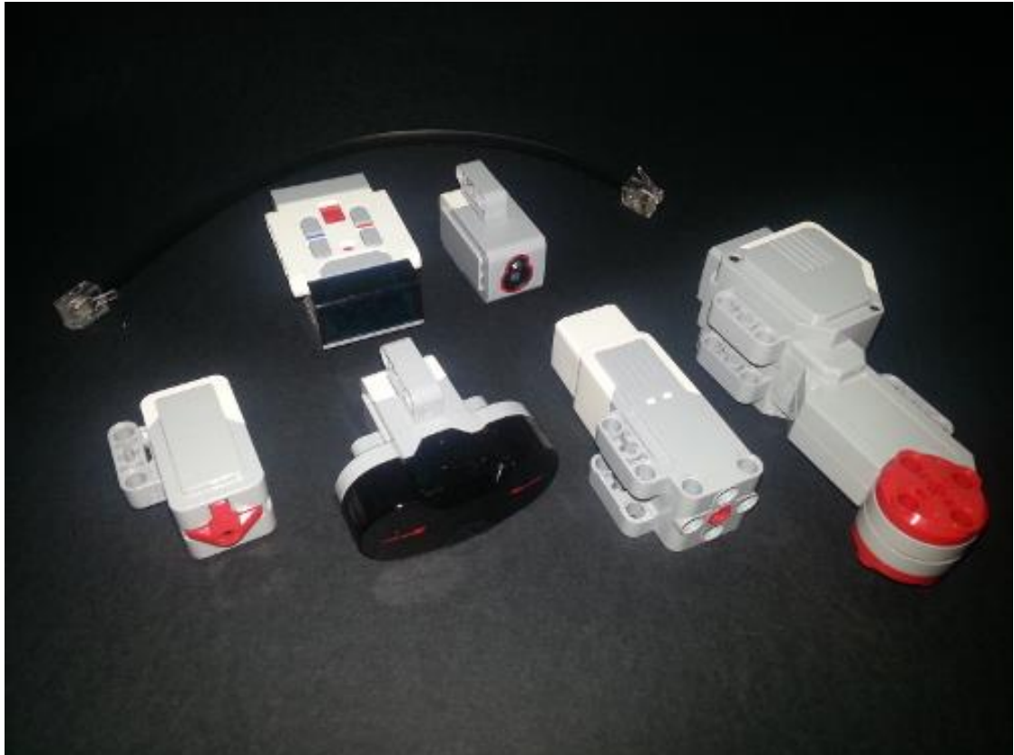
FIGURE 6. Sensors and motors coming in the EV3 home set. From lower left to right: touch sensor, infrared sensor, medium motor and large motor. Up left is a remote control device and next to it a color sensor. On top of them, there is a cable that is used to connect the sensors and motors to EV3 unit
