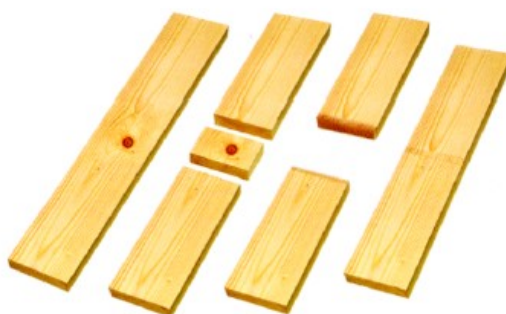
Figure B6-4 Removal of low-value sections and combining via finger-jointing. (Studiengemeinschaft Holzleimbau e.V., 1998)
