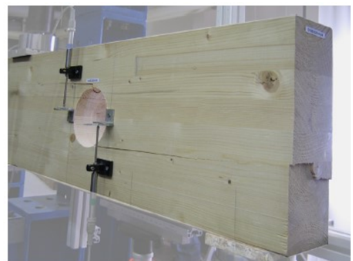
Fig. 14. Shear failure at holes.
