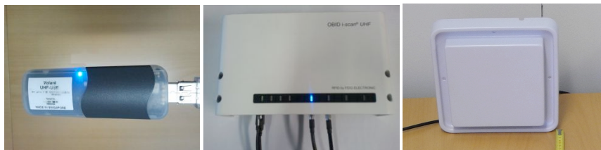
FIGURE 3.2. Left to right: Volare UHF USB reader stick (with an internal antenna), Feig LRU 3500 reader, Feig 270/270mm antenna.
