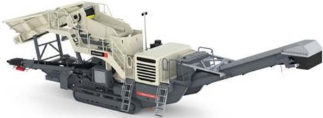
Figure 7. Mobile cone crusher with a pre-screen (Metso Corporation, n.d.-f).
