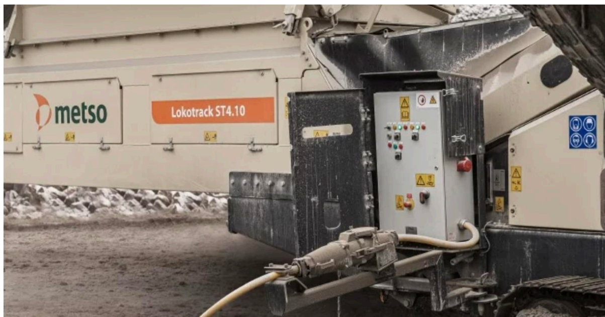
Figure 11. An external power connection for a mobile screen (Metso Corporation, n.d.-l).
