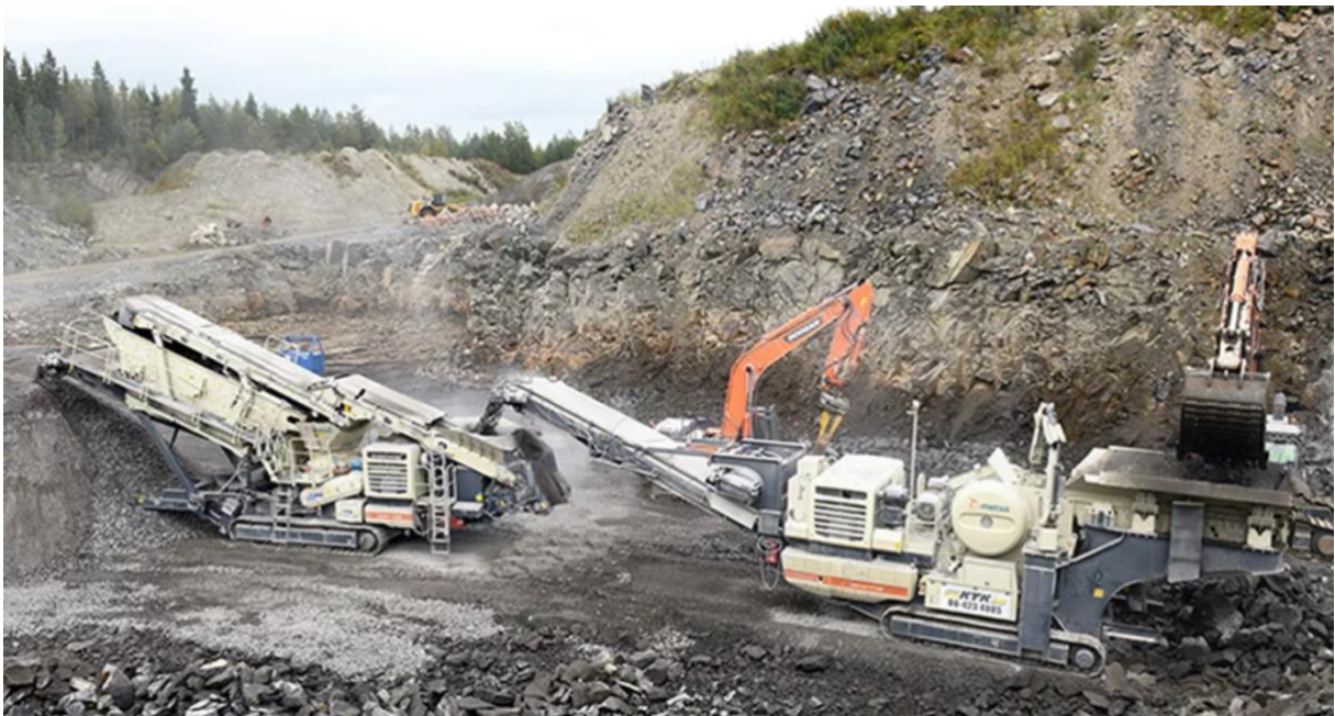
Figure 3. Typical two-stage crushing station (Metso Corporation, 2016).
