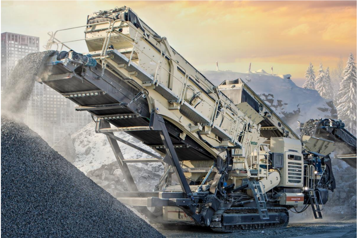
Figure 16. Service platforms of a mobile unit (Metso Corporation, n.d.-n).
