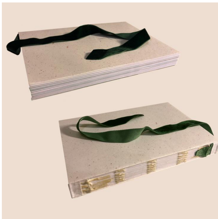
PICTURE 28. Incomplete text block with endpapers and a bookmark but without the mull cloth
