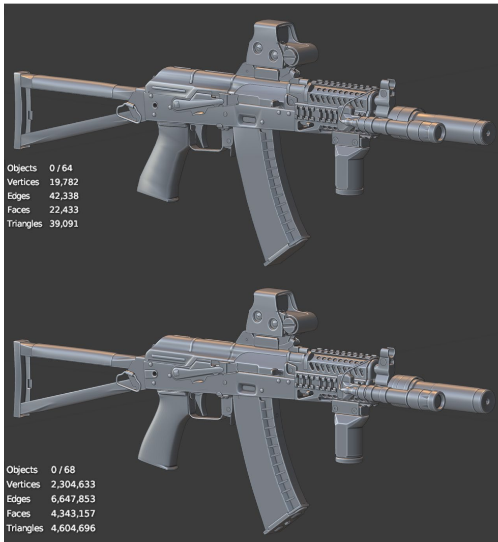
Figure 4. A low poly on top and high poly on the bottom with statistics
