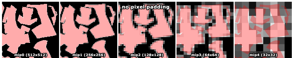
Figure 21. A 512x512 texture down sampled progressively (Polycount Wiki 2017)
