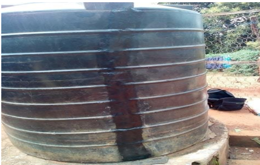
PICTURE 4. A repaired plastic tank using other plastic waste (Restore,2023).
