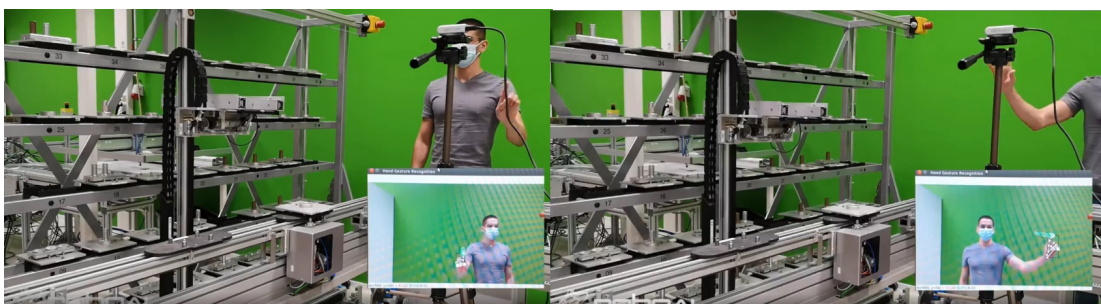
Figure 32: iCIM robot controlled by hand gestures
