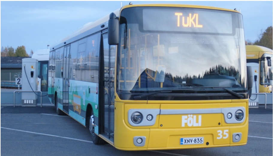
Figure 8. At time of delivery the buses needed to be reversed to slow charging due to placement of the CCS plug. The metal fence visible in the background causes a risk of collision. (Markku Ikonen)
