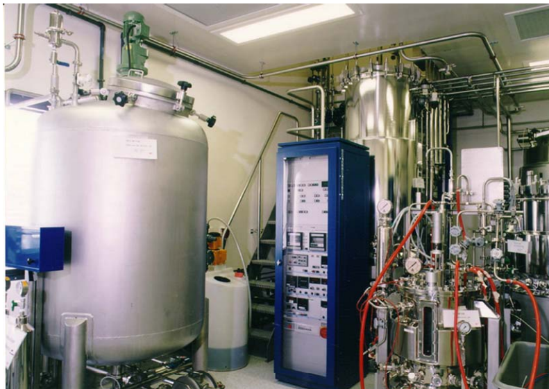
Figure 3: Un-cleanable bioreactor by congestion and poor design
