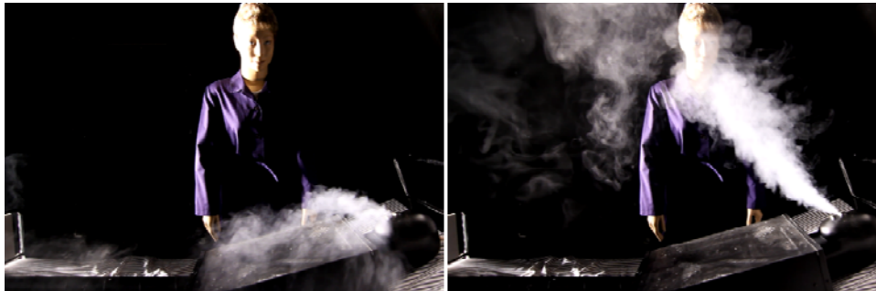
Figure 2. Smoke visualizations of the dispersion of the patient exhaled air. The case with local downward supply is shown on left and with overhead mixing on right. The diffusers were placed in the ceiling above the patient in both cases.
