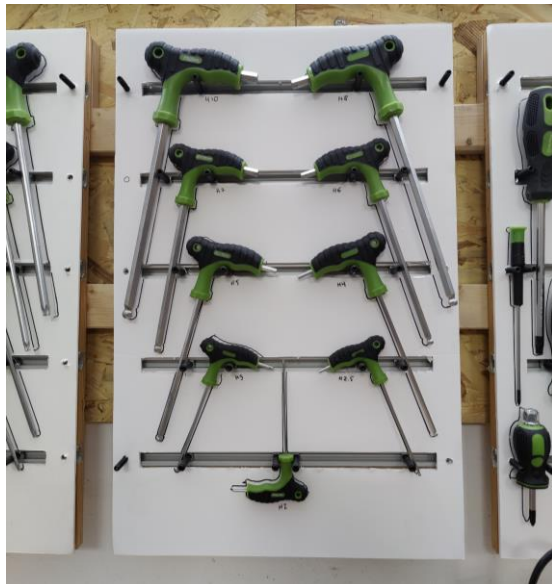
FIGURE 35: A CNC machined wood and aluminium T-slot profiles and mounting with architectural foam board shadows and labelling.
