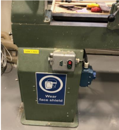
FIGURE 9: Sign reminding to Wear a face shield on the lathe in Construction Workshop. The yellow tape also has the name of the machine in English and Finnish.
