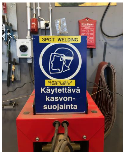
FIGURE 10: Construction Metal Workshop PPE sign. saying always use a face shield when using the Spot Welder in English and Finnish.
