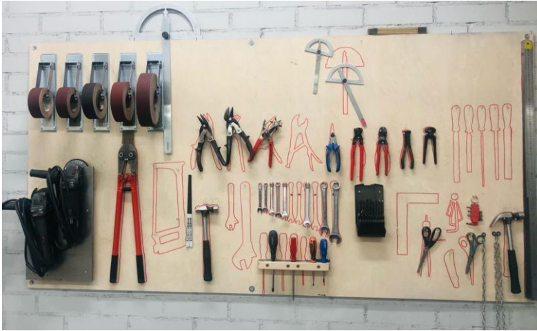
FIGURE 32: Tool wall in Metal workshop in Väre. Outlines clearly indicate which tools are in use or missing. Also notice that some tools are placed in the wrong area.
