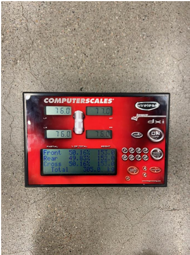
Figure 11. HPF023 corner weights with 85 kg driver.
