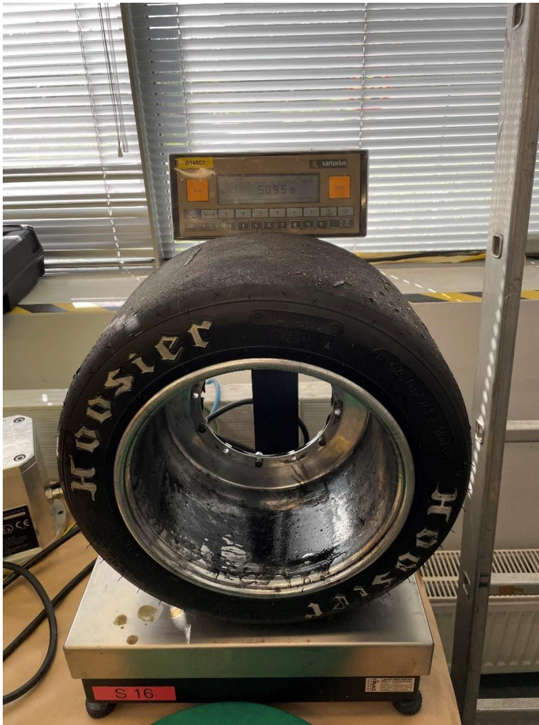
Figure 13. HPF023's wheel on the precision scale.
