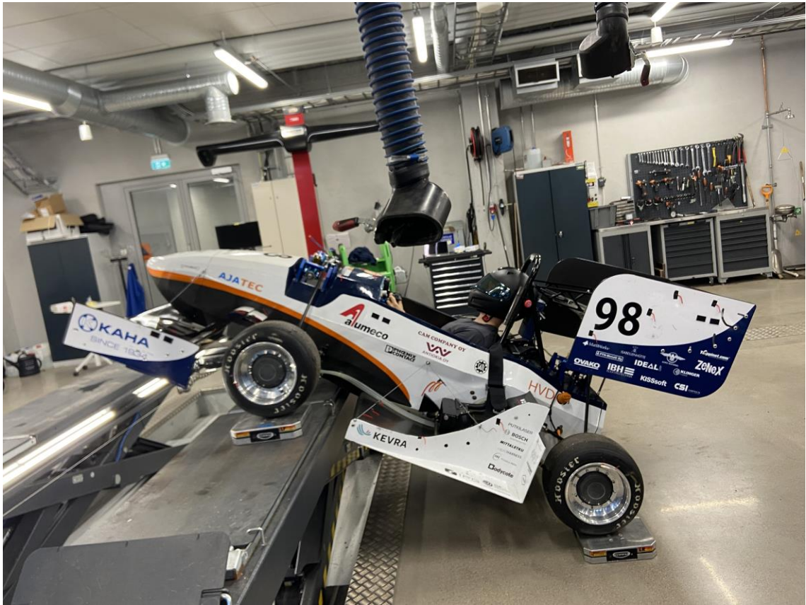
Figure 12. HPF023 during COG measurements.
