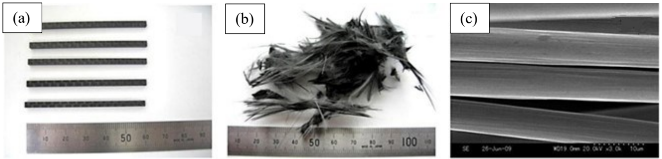
PICTURE 7: Appearance of recovered carbon fibre at 270 °C, 8 MPa and 90 min: (a) CFRP before decomposition, (b) recovered carbon fibre after decomposition, and (c) SEM photo of recovered carbon fibre (magnification: 3000x), from the batch reactor (Adapted with permission from Okajima et al. 2014, 68—76. Elsevier).
