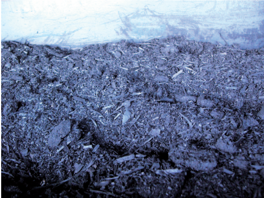
Figure 2. Biochar produced from horse manure in sawdust bedding (Photo: Tomi Holstila).
