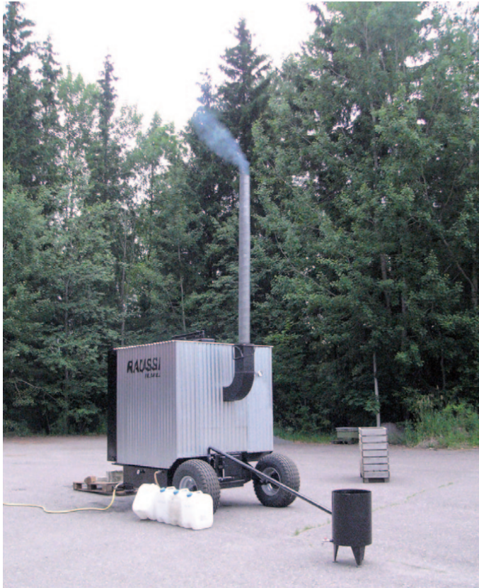
Figure 1. MTT demonstration scale mobile pyrolysis retort (Photo: Tomi Holstila).
