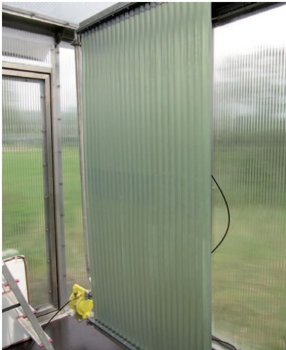
Figure 5. This reactor shows light green from micro algae after two days (Photo: Anne Ahtiainen).
