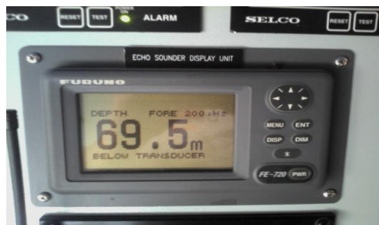
Furuno FE-720 is the repeater of the master unit FE-700.
