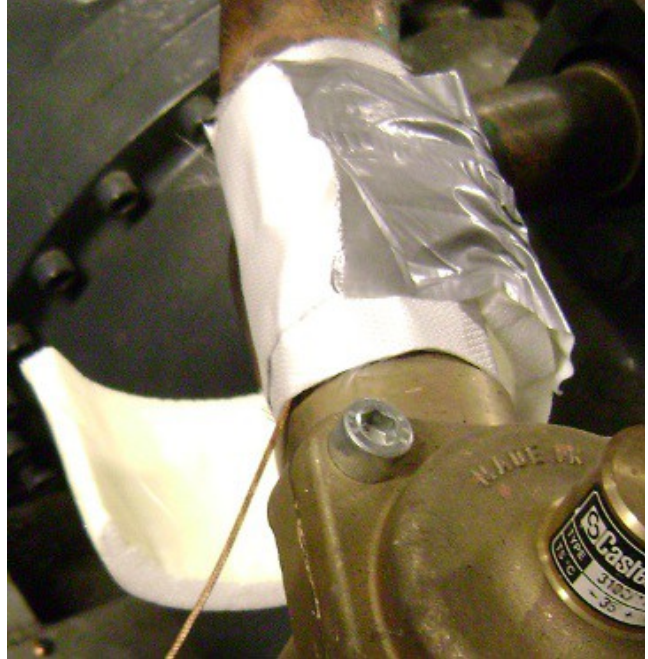
Figure 8: Sensor placement with heat insulation and insulation from room air;
