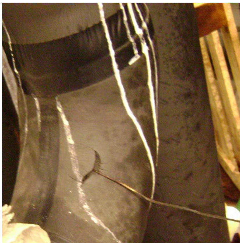
Figure 4: Destructive sensor placement; source: KyAMK EnergyLab
