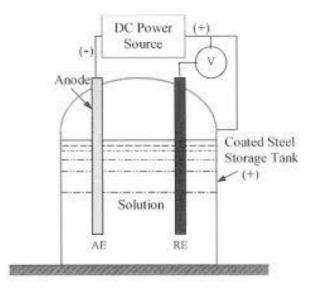
Figure 20: Anodic Protection (Perez, 2004)
