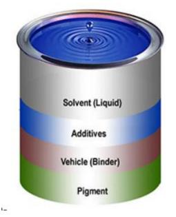
Figure 18: Common components in a coating. (Dean, 2021)
