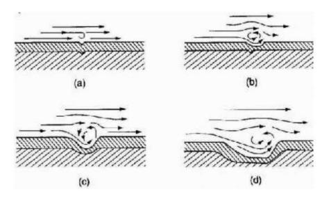
Figure 9: Formation of Erosion Corrosion (Cemmedo, 2015)
