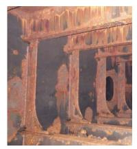
Figure 2: Uniform Corrosion (Estate, 2014)
