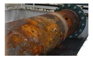
Figure 10: Erosion Corrosion of ship ballast line (Cemmedo, 2015)
