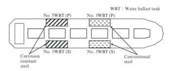
Figure 23: CRS vs Conventional Steel Investigation (Shiotani & Nakamura, 2015)
