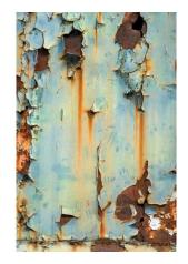
Figure 8: Selective corrosion on shell plate (Moriber, 2020)
