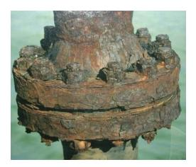
Figure 12: Atmospheric Corrosion of Flange (Flange Band Protectors, n.d.)
