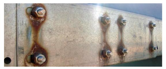
Figure 6: Galvanic Corrosion (Wheeler, 2018)
