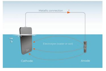
Figure 21: Sacrificial Anode Protection (Cathwell, 2023)
