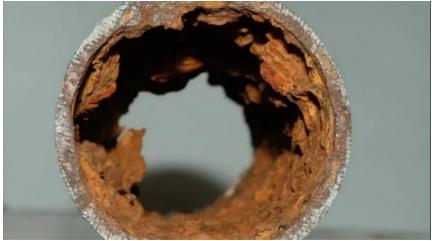
Figure 14: Microbiological Influenced Corrosion (Rope, 2020)
