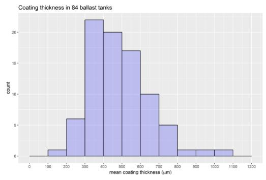
Diagram 2: Average thickness measured. (Willemen et al., 2020)
