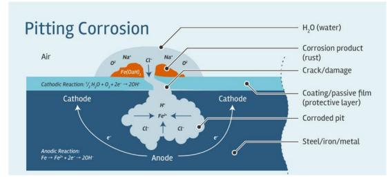
Figure 5: Formation of Pitting Corrosion (Coatings, 2016)
