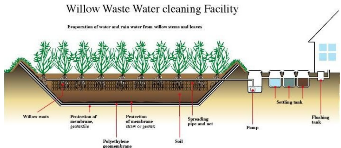
Figure 6. A willow treatment system with zero-discharge. The treatment area is isolated from its surroundings thus causing no leaching to the ground. Water is eliminated through evaporation. /17/
