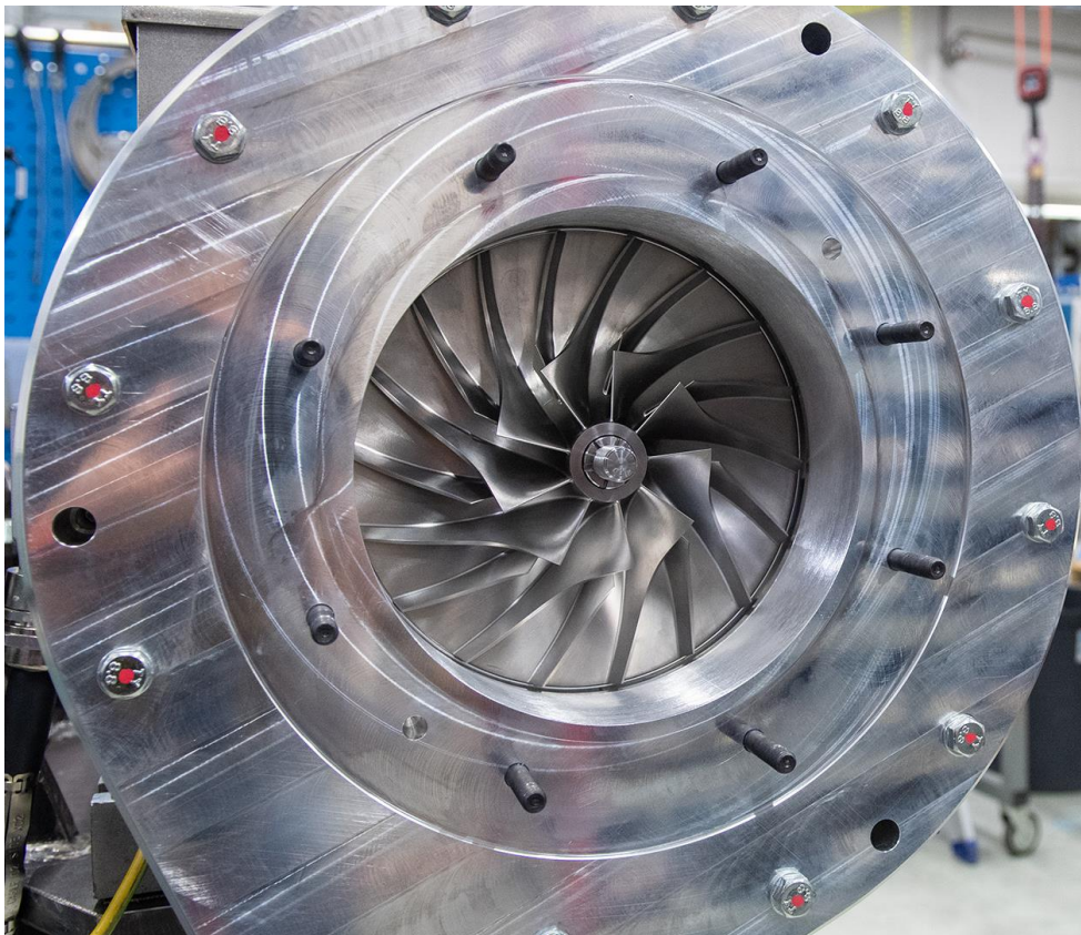
PICTURE 2. An impeller and a turbo frame. (Evolution magazine from SKF 2023).
