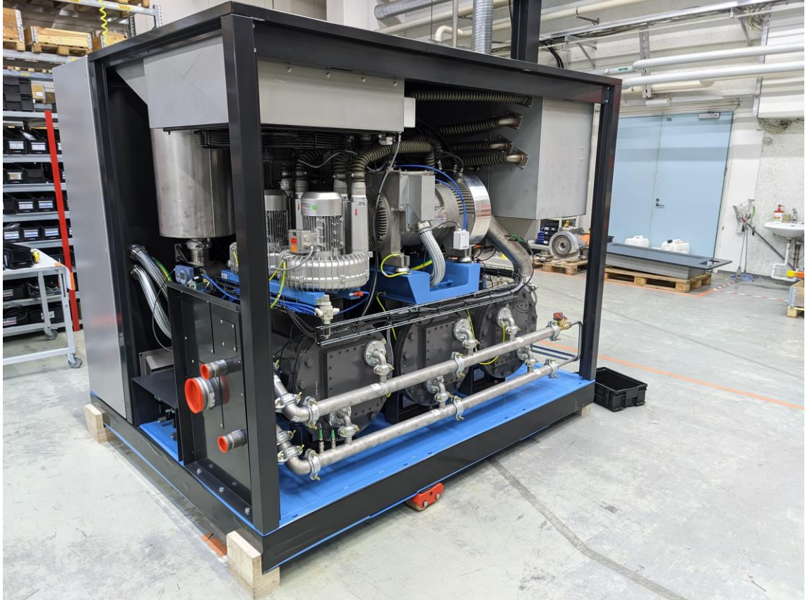
PICTURE 4. Tamturbo's TT325 air compressor (Picture: Lahti 2023).
