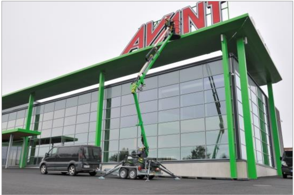
PICTURE 2. A Leguan 125 being operated off a towable trailer at the Avant factory (Photo: Avant Tecno Oy 2011)
